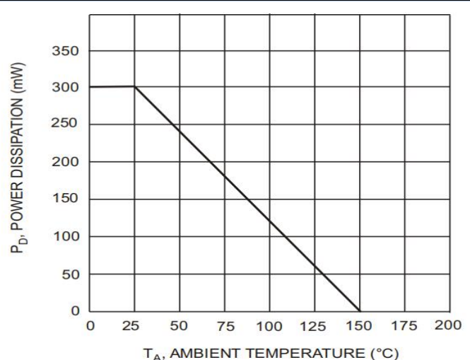
Fig.6 Power Derating Curve
