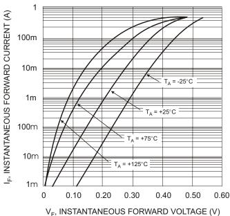
Fig. 2 Typical Forward Characteristics
