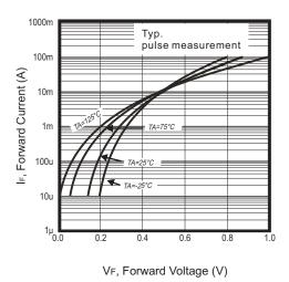
Fig.1 Forward Characteristics
